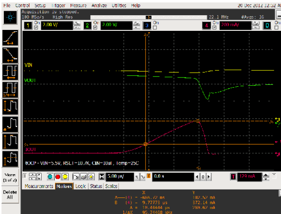
Figure 11. t_{OCP} Response Time
