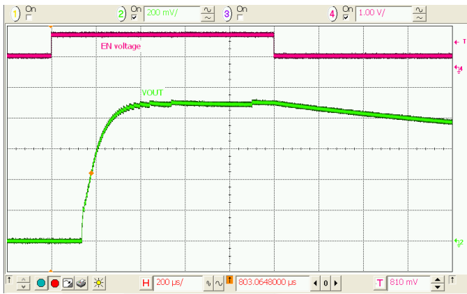
Figure 30. Startup / Shutdown, No Load, V_{OUT}=0.9\text{ V}
